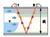
$Q = f(\emptyset 1.t12.t21)$  $\Delta t = t21 - t12 = Kv$ with K: proportion coefficient
