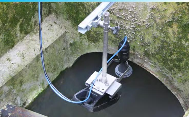
Non-contact RADAR flow measuring system
