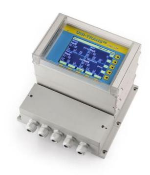
The UNI-TRANSTM is a universal monitor interfacing with multiple sensors and sensor combinations by using up to four RS485 digital serial interfaces with specific communication protocols for the new generation non-contact radar velocity RAVEN-EYE® sensors and ultrasonic transittime FLO-SONICTM sensors, up to eight analog inputs (0/4-20 mA) and up to eight digital inputs or any combinations of those.
